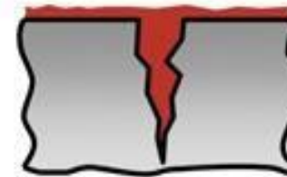
3 Application of penetrant
